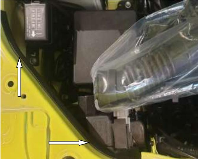
35. Fit pinch weld to radiator support panel as shown in photo.
