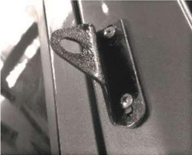
26. Remove the door pillar bracket from the snorkel body (retaining the fastener) and secure the door pillar bracket in place on the A-pillar using 3/4" x 8G stainless steel PK screws (2).
