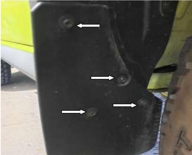
6. Remove and retain the fasteners that secure the RHS mud flap in place.
