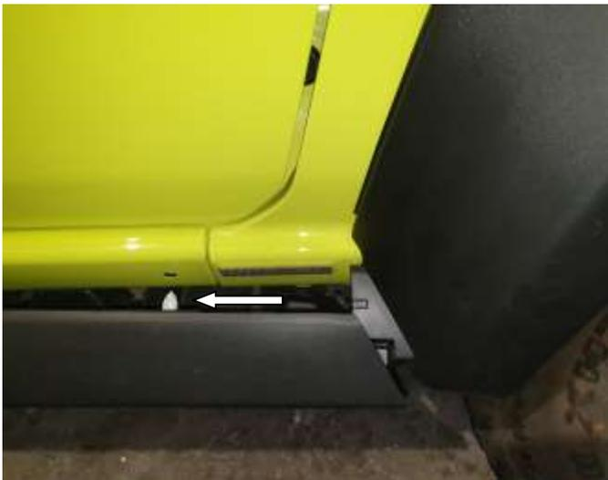
7. The side plastic sill cover will require the fasteners to be un-clipped out of the sill panel.
