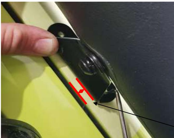
21. Using the bracket as a template mark the two-hole positions on the A pillar.
