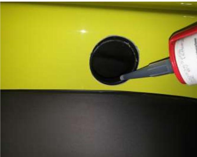
28. Apply a neutral cure silicone to the inside of the tube section of the intermediate tube.
