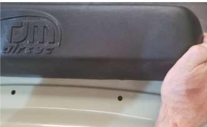
31. Secure the snorkel body in place using M8 x 1.25 nyloc nuts (5), 5/16" x 1-1/4" flat washers (5).
