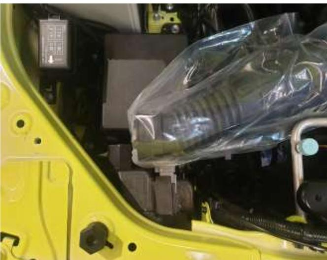
5. Cover the engine intake pipe with a clean plastic bag or similar so no foreign matter can enter the engine
